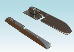
Building upon the popularity of the H25-0023 heavy-duty Command Ratchet Hinge, this new 18-1/2" hinge features a hard stop at 105° and is ideal for longer seat backs up to 22". This extended specialty hinge features one locking position at 62.5° and is perfect for sun pads, bolsters and lounge backrests.
