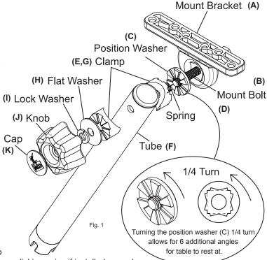
round position washers in the same position. You should here a clicking noise if installed properly.
