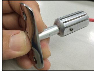
View of LED being slid out of heatsink and cover plate
