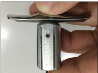
View of how best to hold heat sink and cover plate while removing LED
