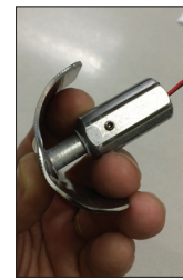
View of LED being slid out of heatsink and cover plate
