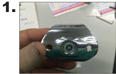
View of assembled navigation light after removal from boat
