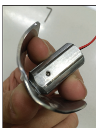
View of how best to hold heat sink and cover plate while removing LED
