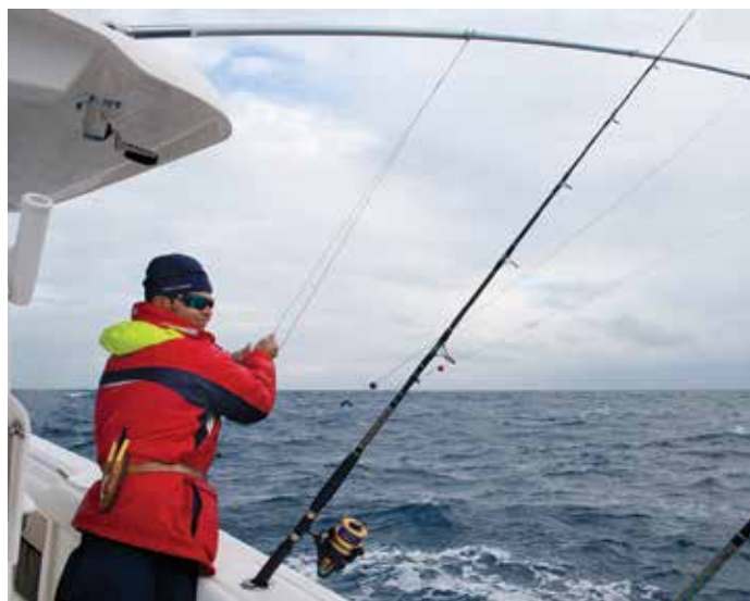
An outrigger mount like the one seen here, under the hardtop, lets you deploy the outrigger pole without climbing on the gunwale to reach the swiveling mechanism. Keeping crew members inside the boat is a safety benefit, especially when seas are rough.
