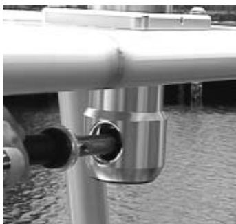
Align handle making sure not to lose nylon bushings, then tighten nut
