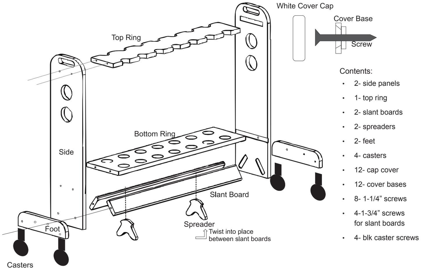
1. Attach bottom ring to side panels using 1-1/4" screws, caps & cover base.
